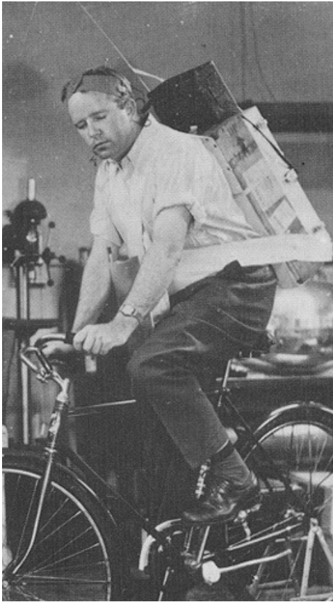
Wikipedia. The original Holter biotelemetry apparatus in 1947 weighing 85 lb
